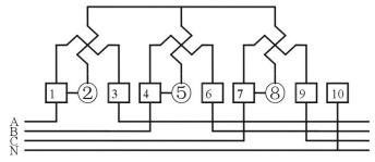
(2) three phase four wire through current transformer connection
