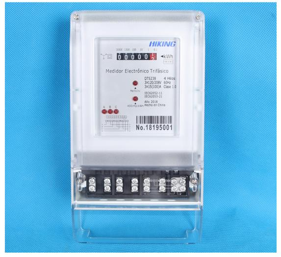
The meter is used in three phase four wire power grid. The meter is designed to measure AC active energy. All of its functions comply with the relative technical requirement for class 1 three phase watt hour meter in IEC62053-21. It is a long life meter with the advantage of high stability, high over load capability, low power loss.
