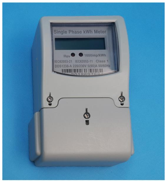
The meter is designed to measure single phase two wire AC active energy. It adopt LSI and SMT technology, the key component are long life international brand product. All of its functions comply with the relative technical requirement for class 1 single phase watt hour meter in IEC62053-21. It is a long life meter with the advantage of high stability, high over load capability, low power loss and compact size.
